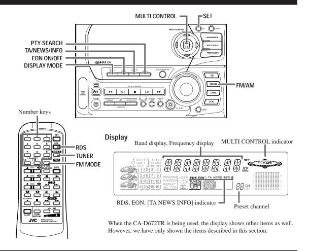
You can listen to both FM and AM (MW/LW) stations. Stations can be tuned in manually, automatically, or from preset memory storage.
